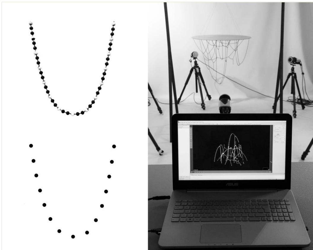
Figure 10: Motion capture is performed using reflective markers placed on the chains (left). This recording system enables the real-time observation of the funicular model on the computer (right).
