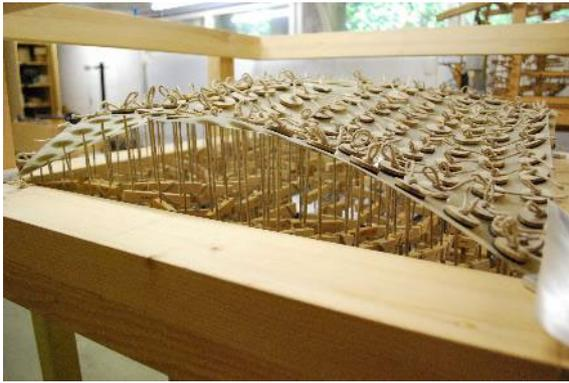
Figure 7 Physical model demonstrating potential edge buckling of the Heimberg shell at midspan (Photo: John Chilton)
