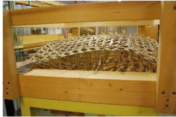
Figure 8 The same physical model showing an alternative potential buckling mode of the Heimberg shell (Photo: John Chilton)
