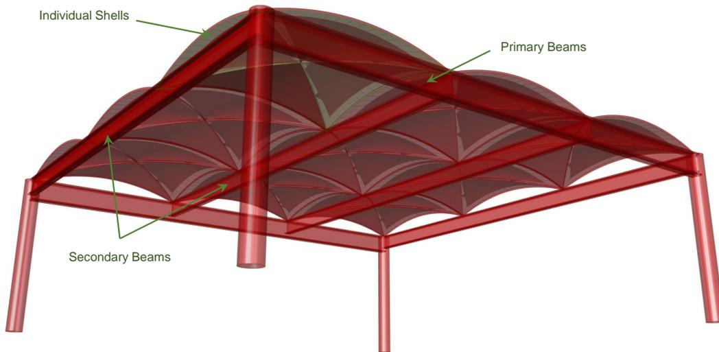
Figure 1: Composite floor system with individual shells supported by a beam grid.
