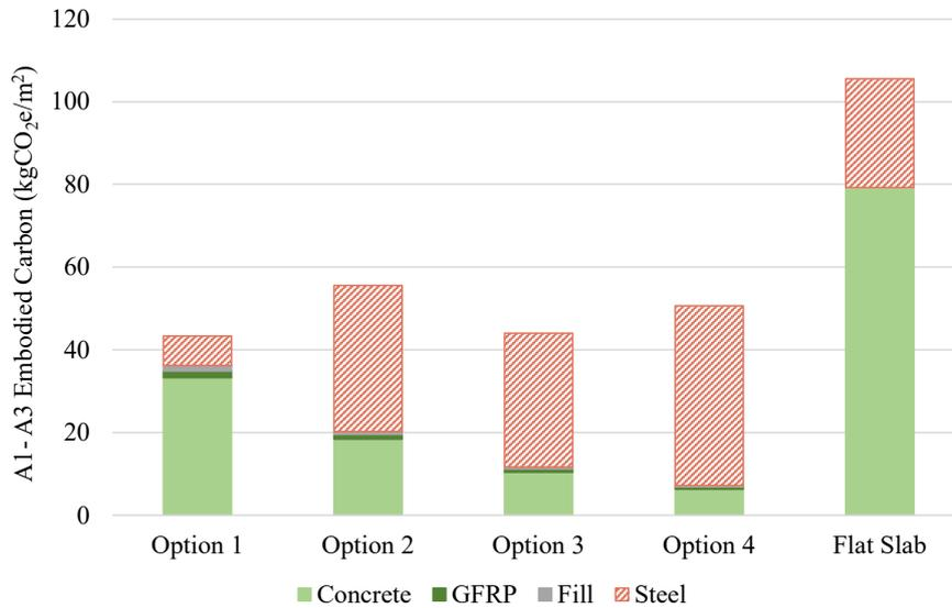
Figure 4: Embodied carbon of different floor options.
