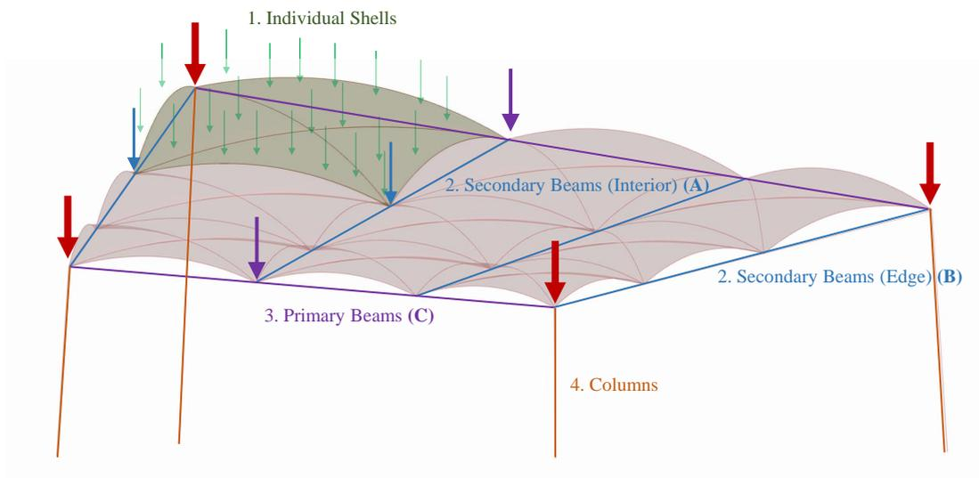
Figure 3: Elements in the proposed composite floor system.
