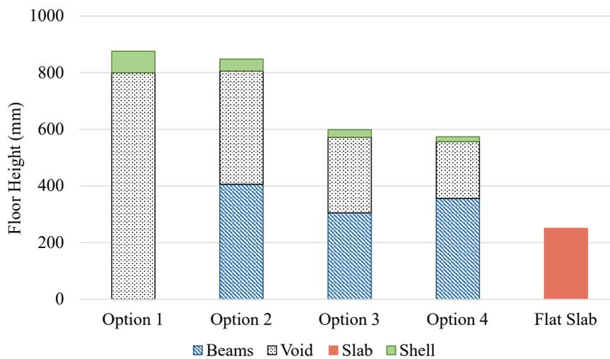
Figure 5: Floor height of different floor options.
