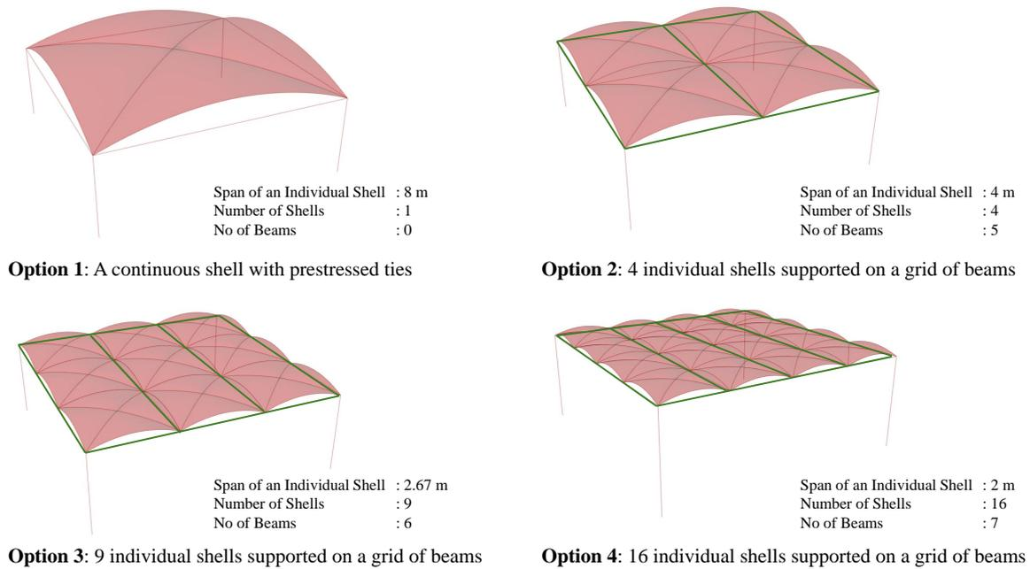
Figure 2: Variations of the shell-beam composite floor system.
