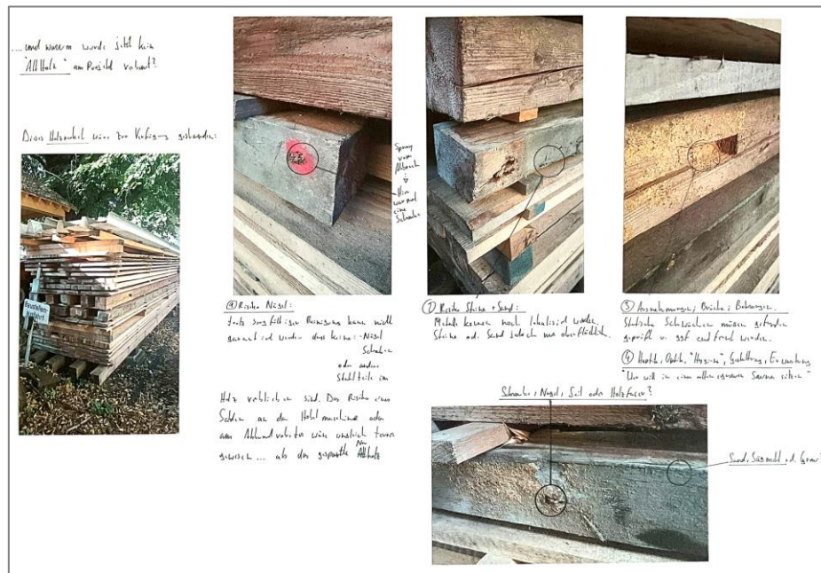
Figure 6: Screws, stones, sand and dirt: While metallic contaminants can be localized and removed with a metal detector, this is not possible for sand and stones. The risk of machine damage when using reclaimed wood on the joinery robot was ultimately too great for the carpentry company.
