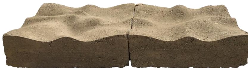
Figure 3: A RE modular block rammed on site by the author in a previous study. (Image provided by and reproduced from [16])
