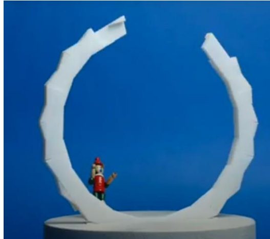
Figure 6 Scale model of the interlocking blocks during assembly, 3D printed in PLA https://youtu.be/a3v0kSaaMJE
