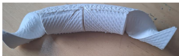
Figure 7 Three interlocking blocks with a spiral shape. 3D printed in PLA.
