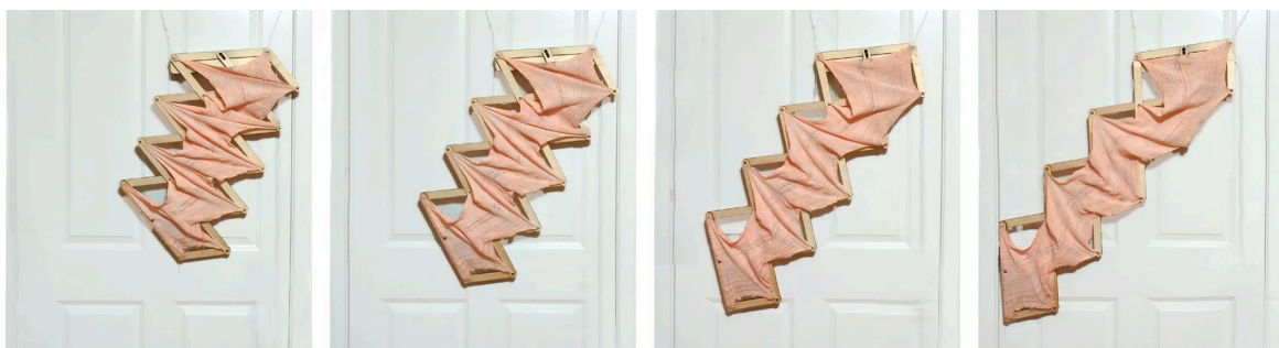
Figure 13: Arduino and servo motor automated scissor structure with loose knit [Image source from author]
