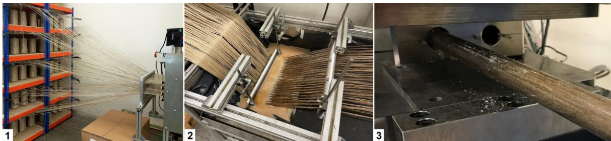
Figure 1: Pultrusion process: (1) Natural flax fiber rovings, (2) fibers being impregnated into the matrix, (3) cured pultruded profile \varnothing 25 mm exiting the heated mold
