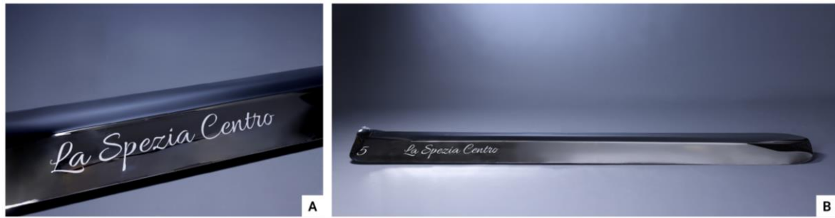
Figure 6: A) Bead-rolled crease and sandblasted text over the inflated prototype [©Joe Laws Photography] B): The prototype in scale 1:2 of the inflated steel element [©Joe Laws Photography]
