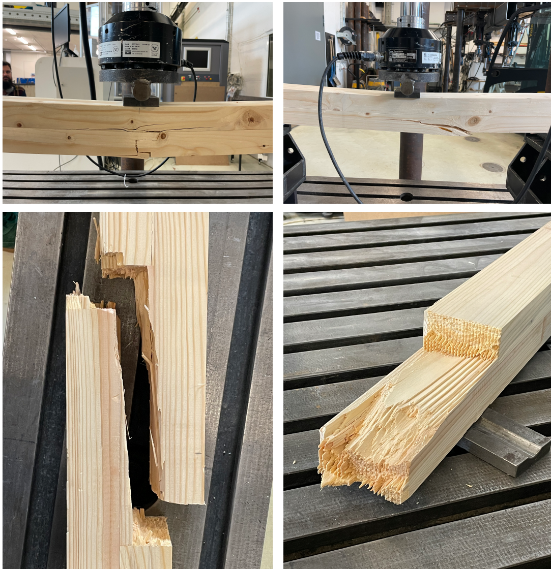
Figure 7: The structural testing showed that breakage starts in knots and develops along fibres.
