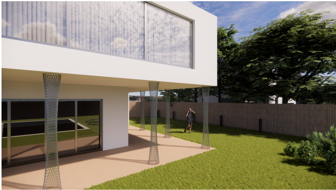
Figure 1: Possible application of WAAM dot-by-dot process to fabricate lattice steel structural elements. Adapted from [23].
