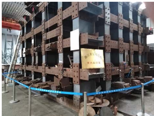
Fig .1 Creep experimental apparatus of steel wire ropes
