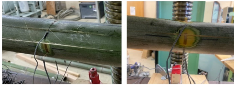
Figure 6: Photos of culm wall bending failure in the bending tests. Left: BT2; Right: BT5.
