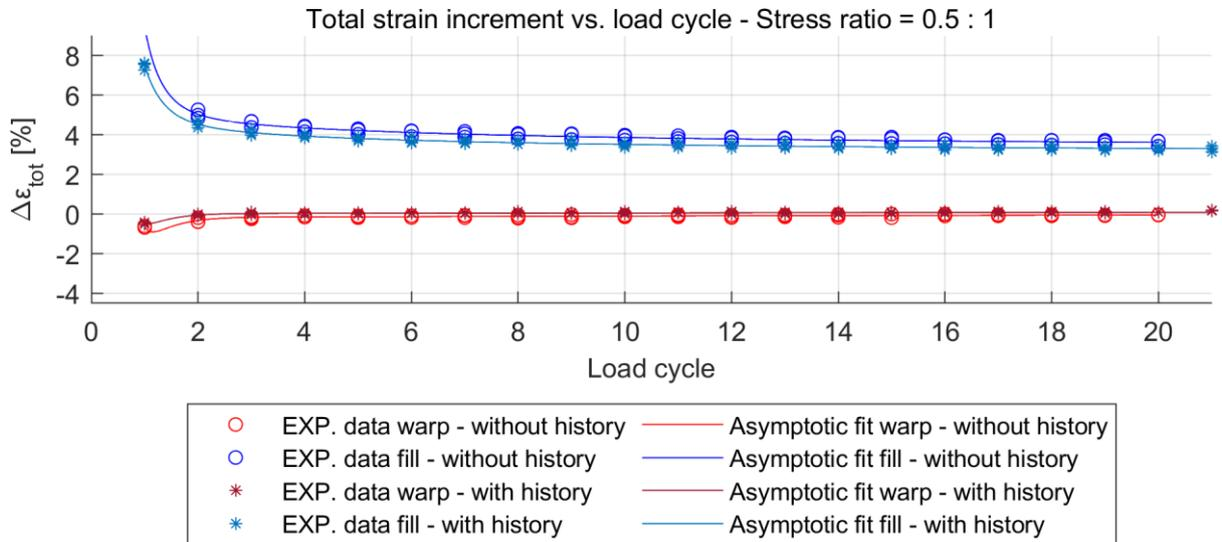
Figure 7: Inspection characteristic total strain  $\epsilon_{tot}$  under stress ratio 0.5:1
