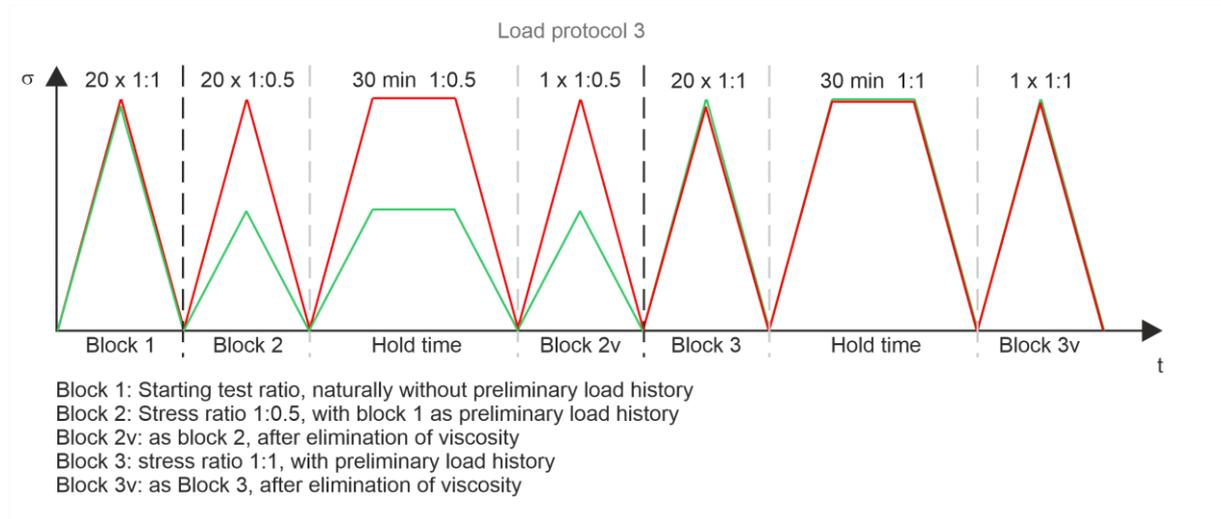
Figure 2: Load protocol with stress ratio 1:1 in load block 1
