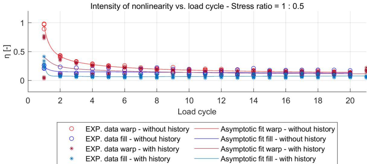
Figure 9: Inspection characteristic intensity of nonlinearity  $\eta$  under stress ratio 1:0.5
