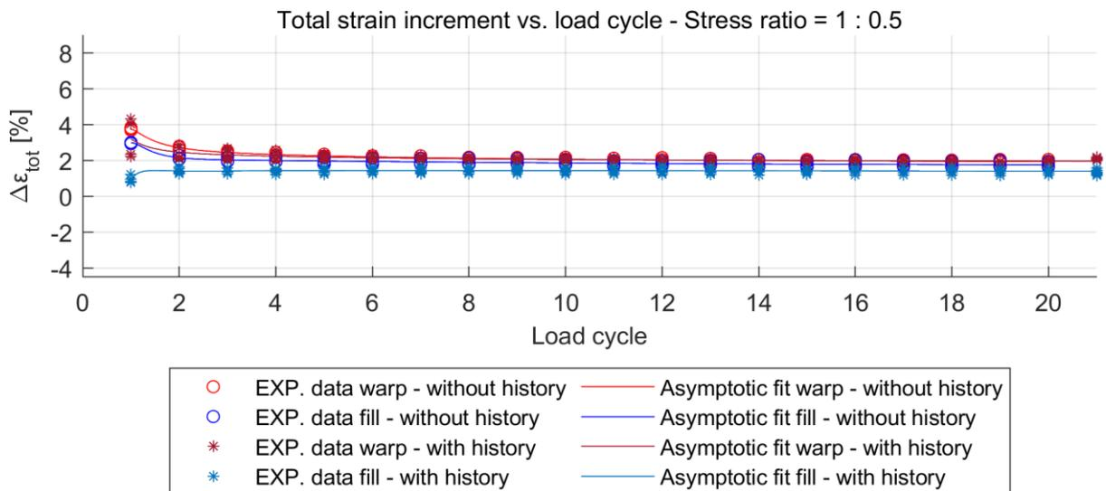
Figure 8: Inspection characteristic total strain  $\epsilon_{tot}$  under stress ratio 1:0.5
