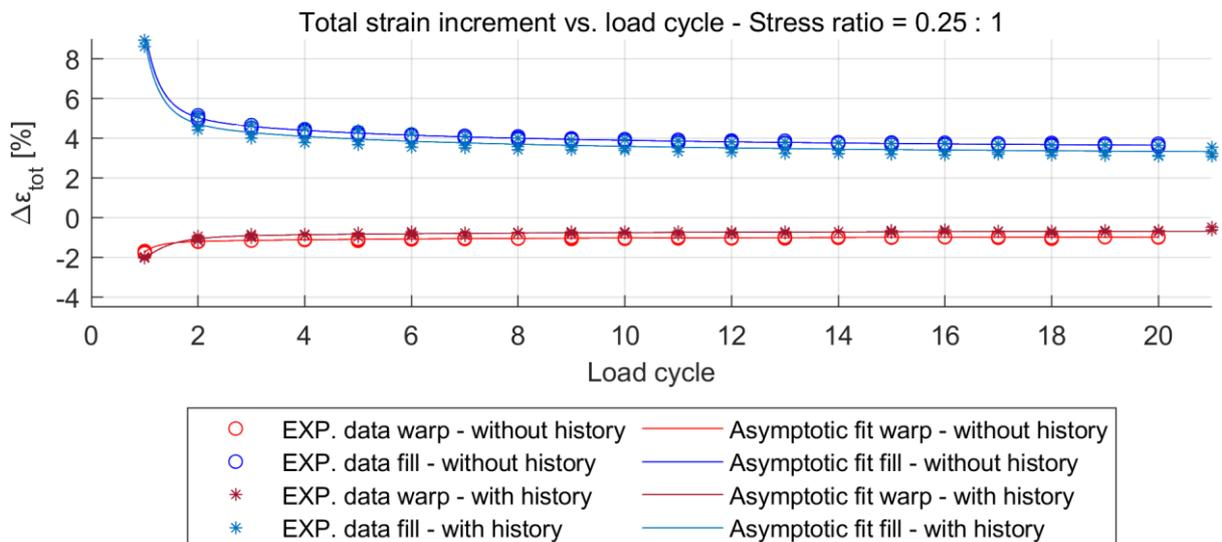
Figure 6: Inspection characteristic total strain  $\Delta\epsilon_{tot}$  under stress ratio 0.25:1
