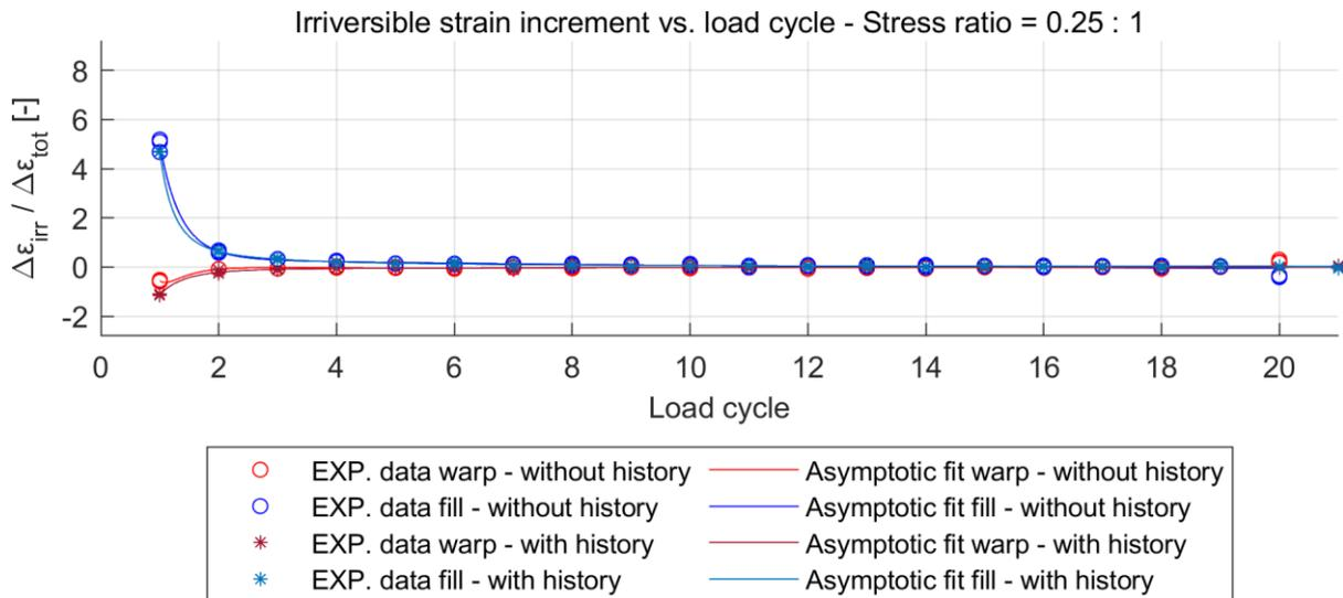
Figure 4: Inspection characteristic irreversible strain  $\Delta\epsilon_{irr}$  under stress ratio 0.25:1
