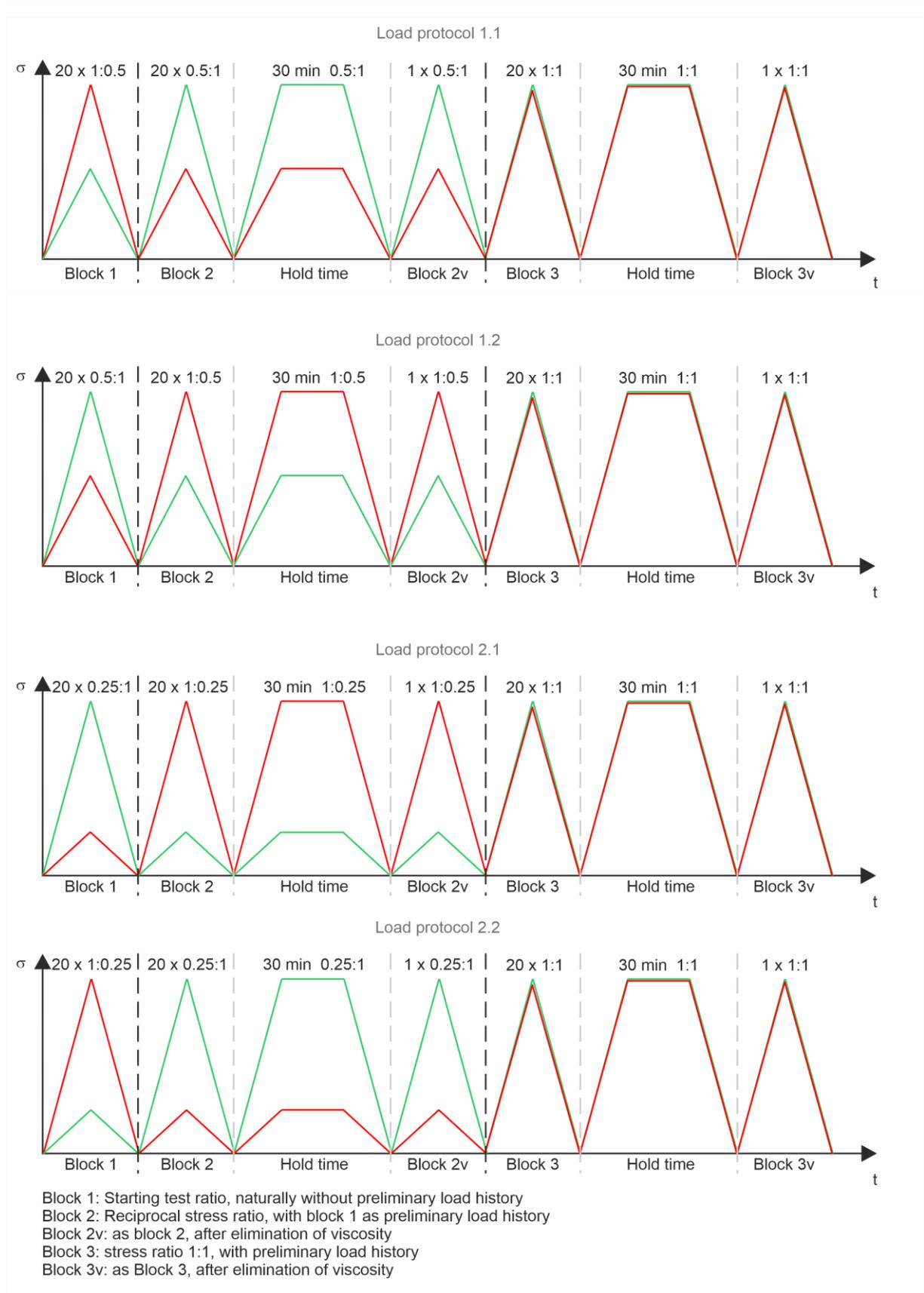
Figure 1: Load protocols with uneven stress ratios in load block 1
