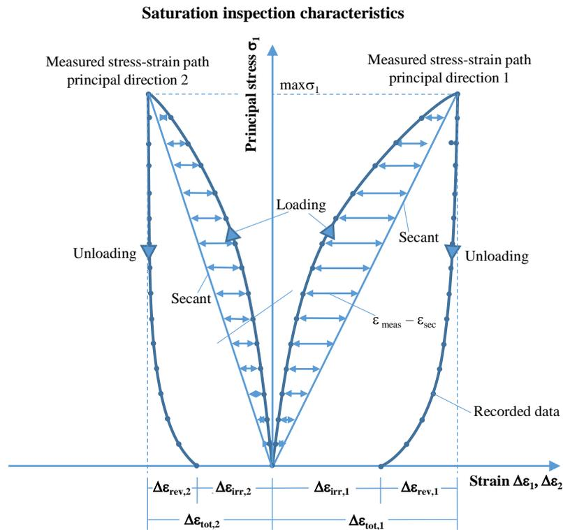
Figure 3: Saturation inspection characteristics ( $\Delta\epsilon_{irr}$ : irreversible strain increment,  $\Delta\epsilon_{rev}$ : reversible strain increment,  $\Delta\epsilon_{tot}$ : total strain increment,  $\epsilon_{meas}$ : measured strain,  $\epsilon_{sec}$ : calculated strain along the secant)
