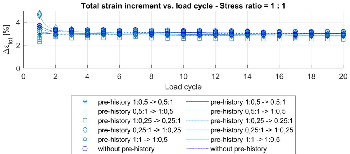
Figure 5: Inspection characteristic total strain  $\Delta\epsilon_{tot}$  for fill direction under stress ratio 1:1
