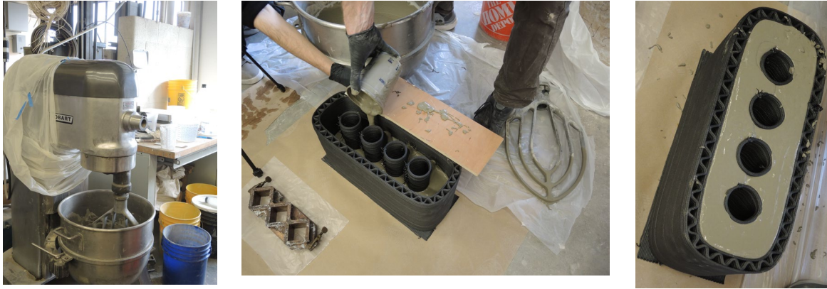
Figure 9. The casting process of the 3D printed formwork; the formwork was strength enough to withstand the wet concrete hydrostatic pressure, with no visible deflection. In addition, no leakage was observed during the casting process (W/C Ratio was 22.5%).
