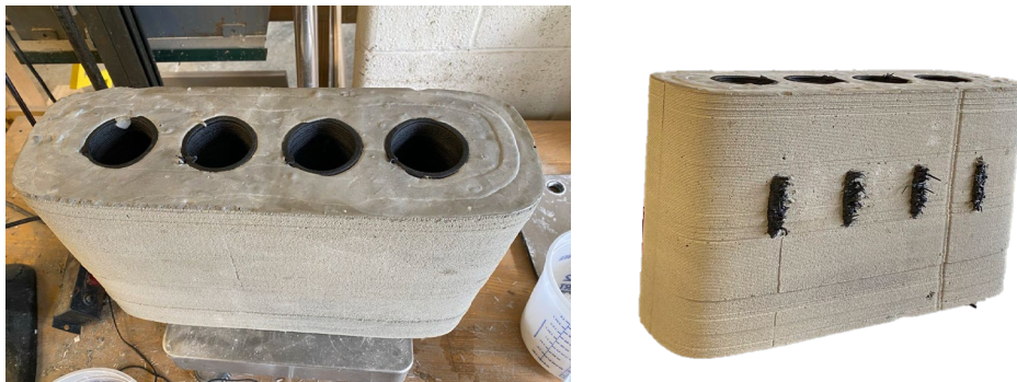
Figure 10. The concrete hollow-core section after demolding; part of the formwork will remain as a lost formwork intentionally (cylinders). The formwork will be ground to be reused. The demolding process did not damage the concrete surface, and the quality of the finished surface is high.
