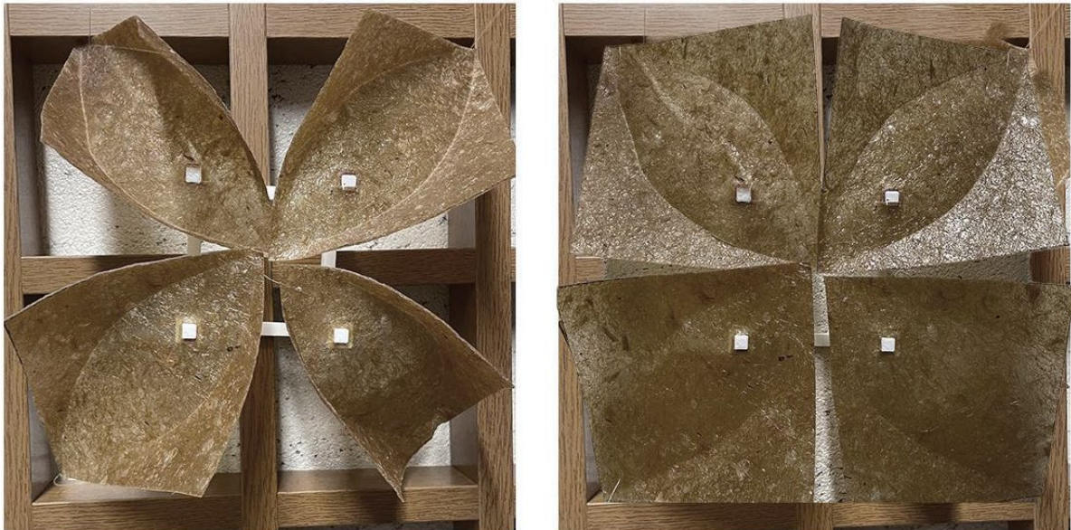
Figure 6. Scaled overall model of the adaptive shading device, open and closed positions
