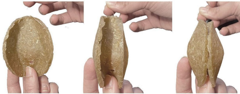
Figure 4. Incapability of S5 to fold and unfold due to its thickness
