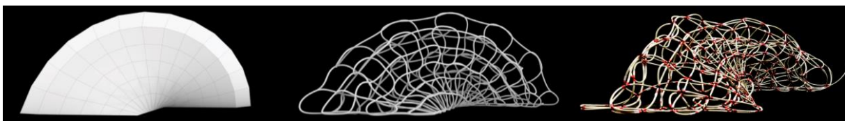
Figure 11: The surface (left), simulation (center), and the physical prototype (right) of a double-layer 3D surface realized by a continuous rod.
