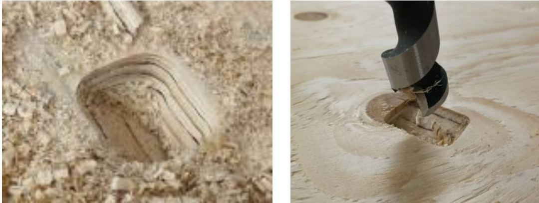
Figure 10: Pilot milling (left); drilling (right)
