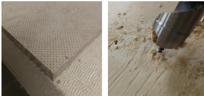
Figure 7: biofibre plate with a homogeneous, rough surface and stainer marks (left); auger on the top layer of an LVL board made of spruce wood (right)
