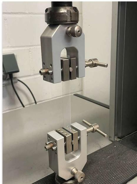
Figure 1: Tensile test set-up with clamping distance of 100 mm.
