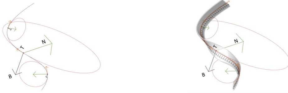
Figure 1: Considering the curve's parameter domain interval between (0,1) , the osculating planes at three points on the curve at [t = 0.25, t = 0.5, t = 0.75] are illustrated. The green arrow represents the normal ( N ), the red arrow represents the tangent ( T ), and the black arrow represents the binormal ( B = T \times N ). The osculating circle with radius R lying on the osculating plane at parameter t defines the curve's curvature K at that parameter, equal to 1/R . The figure on the left shows the profile twist aligned with the curve's binormal vectors at parameter t , based on the osculating plane's rotation.
