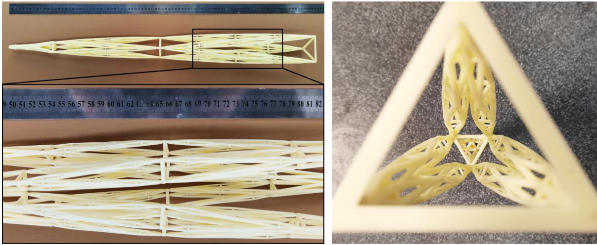
Figure 7: The No.7 hierarchical truss in Figure 6(a) is 3D-printed with ABS using SLA.
