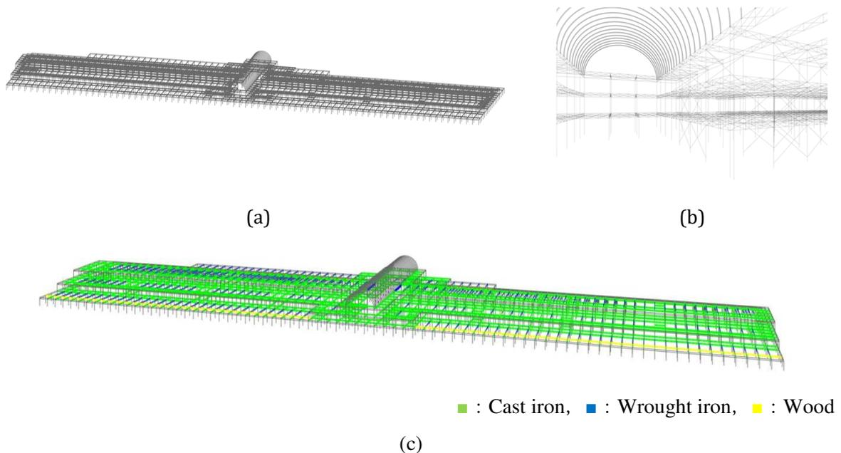
Figure 2: FE model for the Crystal Palace; (a) Exterior perspective view, (b) Interior perspective view, (c) Layout of structural material.
