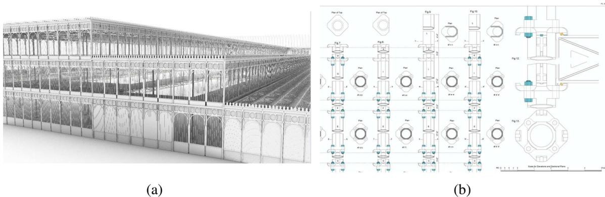
Figure 5: Rigid structural frame, (a) Exterior view of the Crystal Palace on Rhinoceros, and (b) Cross sections of cast-iron columns and details of joint between cast-iron girder and column in PL.8 (traced and colored by third author).
