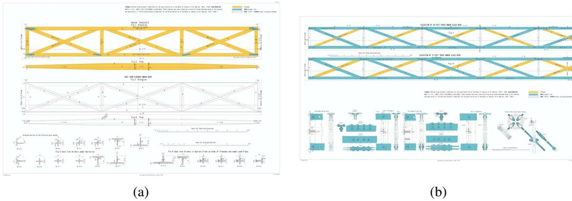
Figure 4: Drawing of truss beams (traced and colored by third author): (a) Wooden truss and cast-iron girder in PL.10, (b) 48-foot and 72-foot truss in PL.11.
