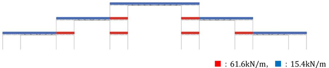
Figure 8: Load condition.
