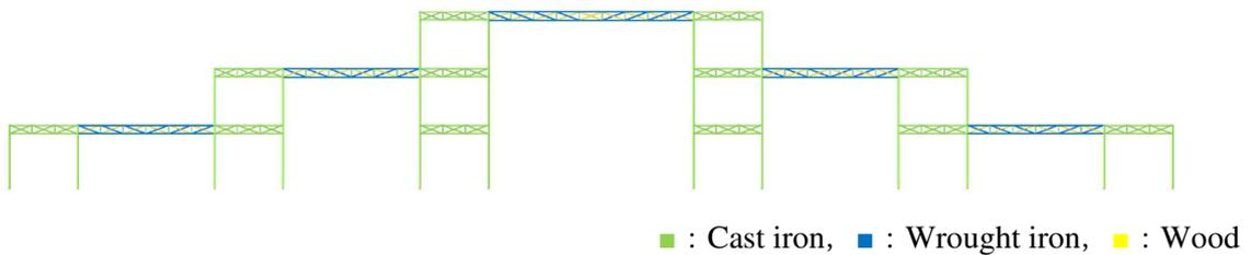
Figure 7: FE model for rigid structural frame in short direction.
