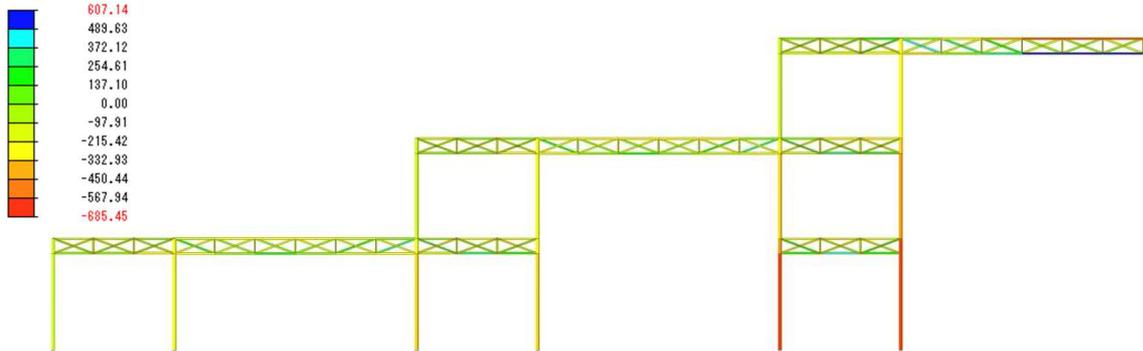
Figure 10: Distribution of axial force against vertical load (Unit: kN).
