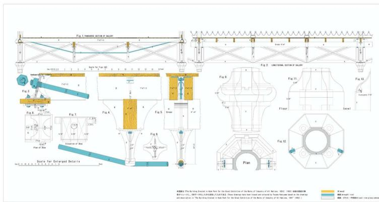
Figure 3: Floor system (slab and joist beam) in PL.14 (traced and colored by third author).
