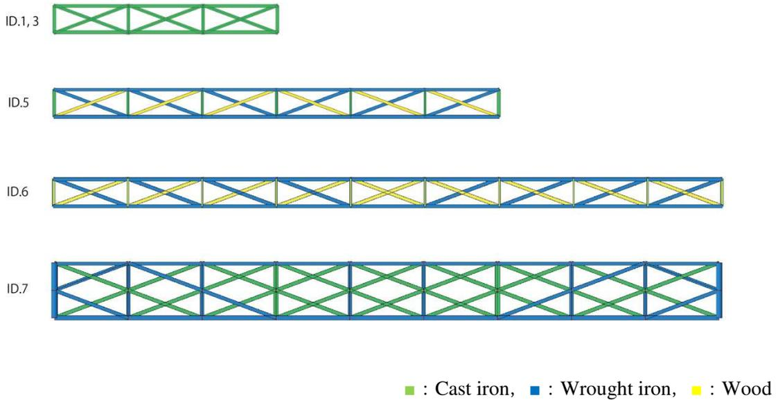
Figure 6: Truss girder with material layout for FE analysis.
