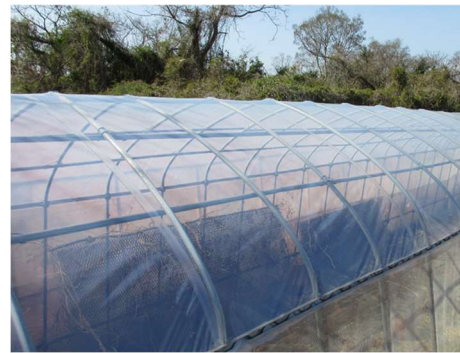
Figure 14 Exposure Test of UV-blocking Film using Silica-coated Zinc Oxide filler.
