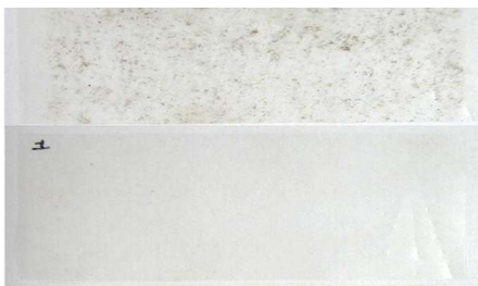
Figure 4 Photograph of a 60 \mu m ETFE greenhouse in use since 1988
