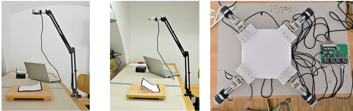
Figure (10): left and middle: scanning procedure with Intel RealSense L515 LiDAR camera; right: uniform stretching with dual-axis membrane testing machine with linear clamping
