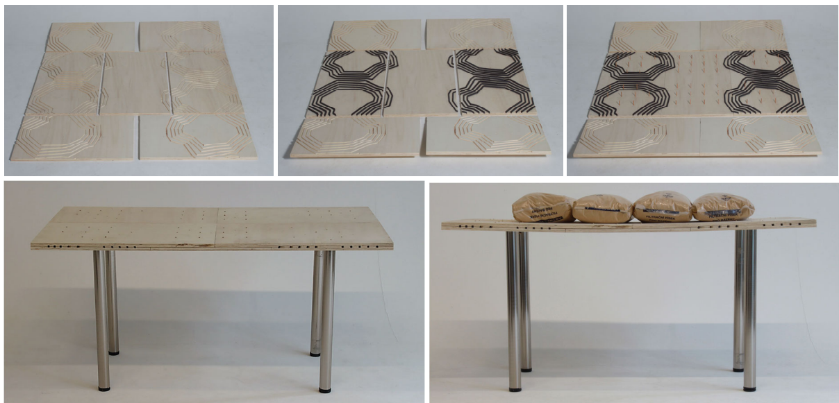
Figure 12: Mock-up: Assembling and testing the construction principle with 100kg of Sand.
