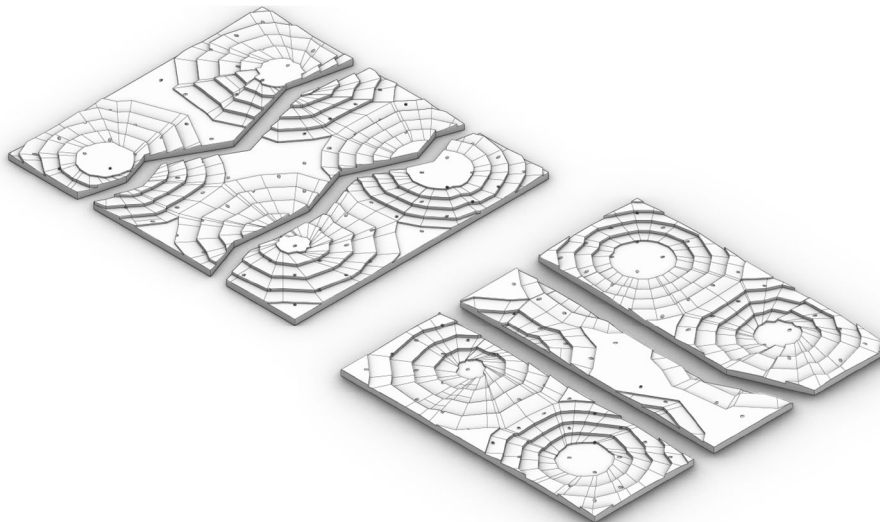
Figure 3: Layers of CLT plates. Left: upper Layer three parts, right: lower layer three parts.
