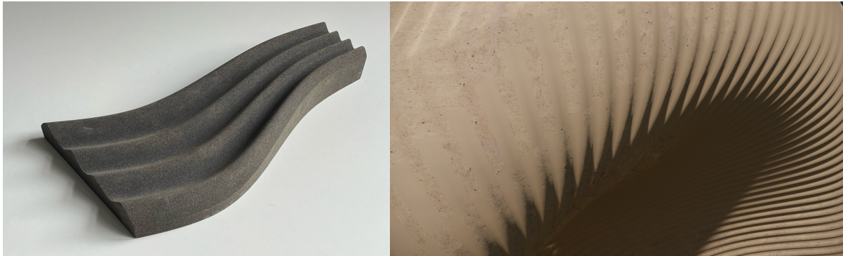
Figure 10: 3d printed formwork negative (left), visualization of texture with pigmented concrete (right)
