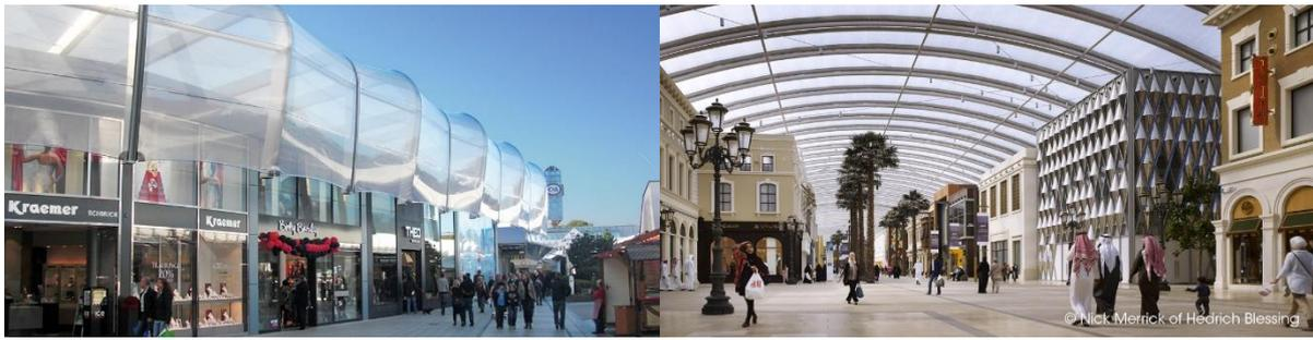
Figure 1: Mechanically and pneumatically prestressed ETFE-foil structures (left: Ruhr Park Bochum, Bochum, Germany, © Taiyo Europe GmbH; right: The Avenues, Kuwait-City, Kuwait, © Nick Merrick of Hedrich Blessing provided by Vector Foiltec GmbH)
