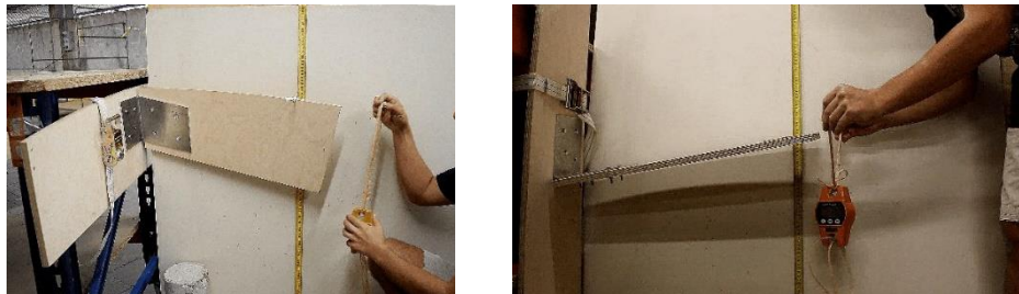
Figure 3: Flat steel plate empirical test applying the load vertically, inward force, horizontal force, down force.
