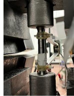
Figure 8: Arrangement of extensometer and strain gauge
