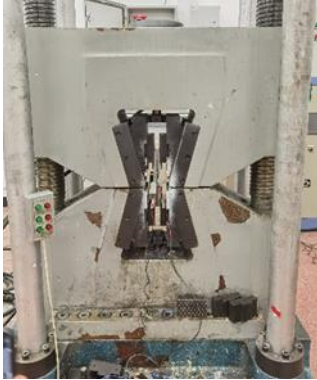
Figure 6: Uniaxial tensile test setup
