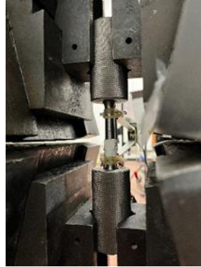
Figure 7: Bolt specimen installation
