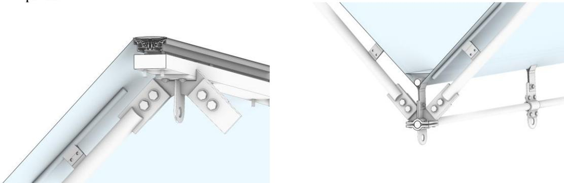
Figure 12: ETFE ridge and valley detail [credit: MAP3 / TAIYO execution drawings]
