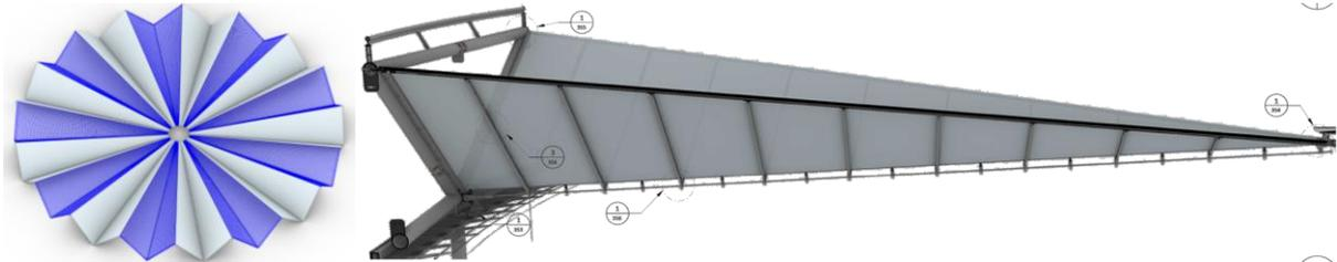
Figure 12: ETFE modules arrangement [credit: T/E/S/S tender package and MAP3 / TAIYO execution drawings]
