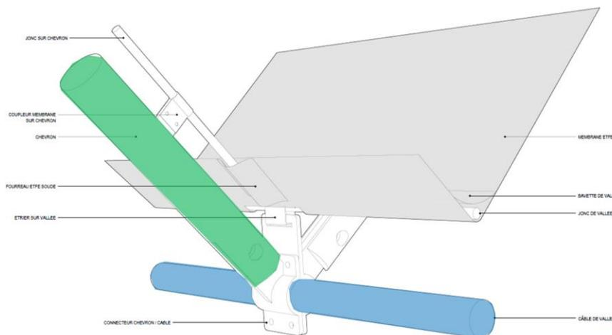
Figure 9 : Axonometric valley details [credit: T/E/S/S tender drawings]
