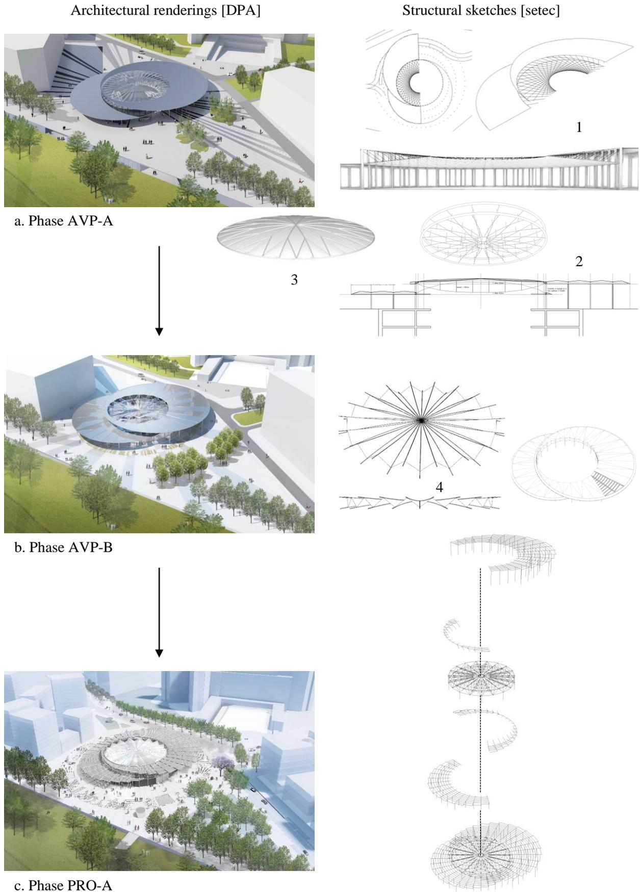
Figure 4: Architectural and structural evolution of the roof during the initial study phases
