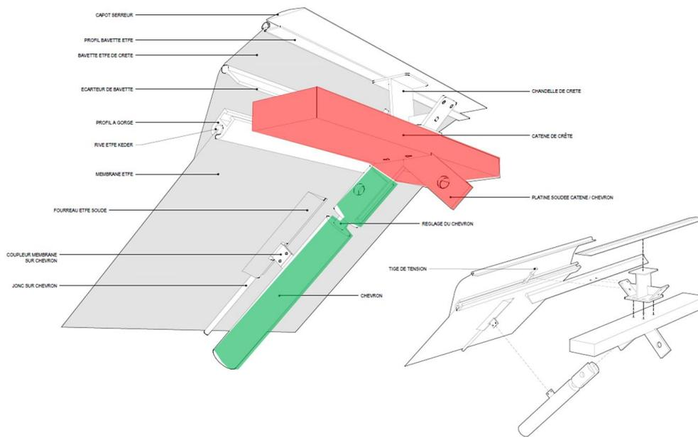
Figure 8: Axonometric ridge details [credit: T/E/S/S tender drawings]
