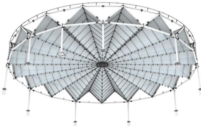
Figure 5: Axonometric view from below of structure and ETFE roof
