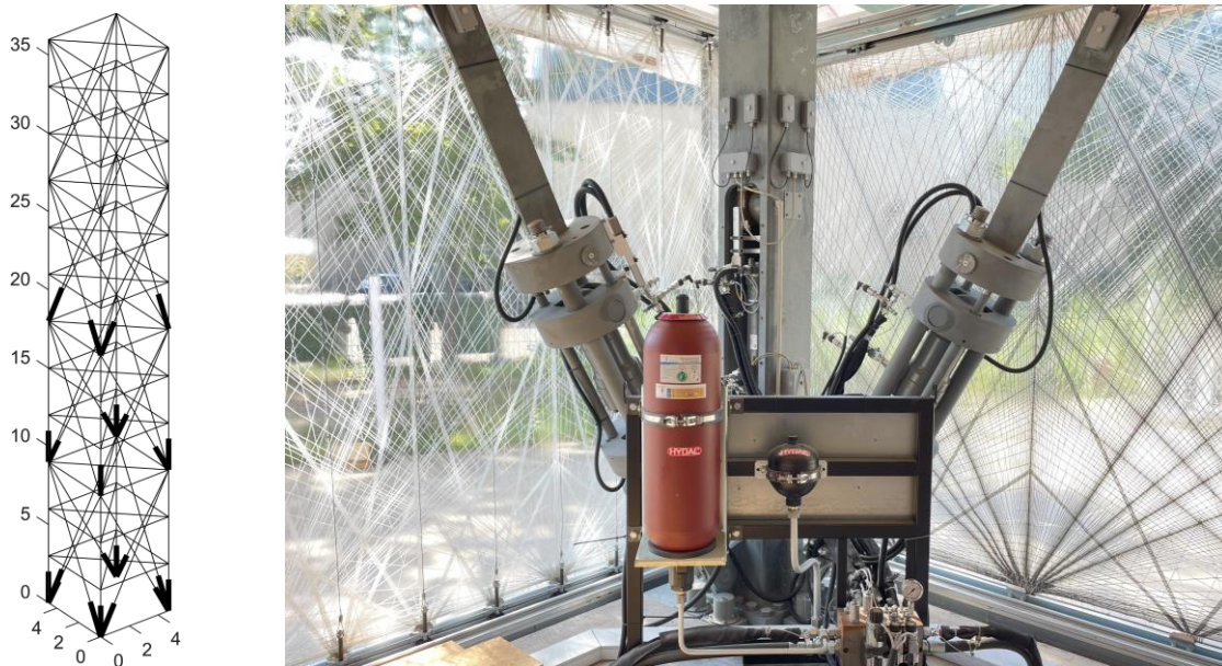
Figure 6: D1244. Left: Actuator placement in the 3D axis model (the bold line indicates the actuators). Right: Actuators and hydraulic system at one corner of the ground floor (© ISYS)
