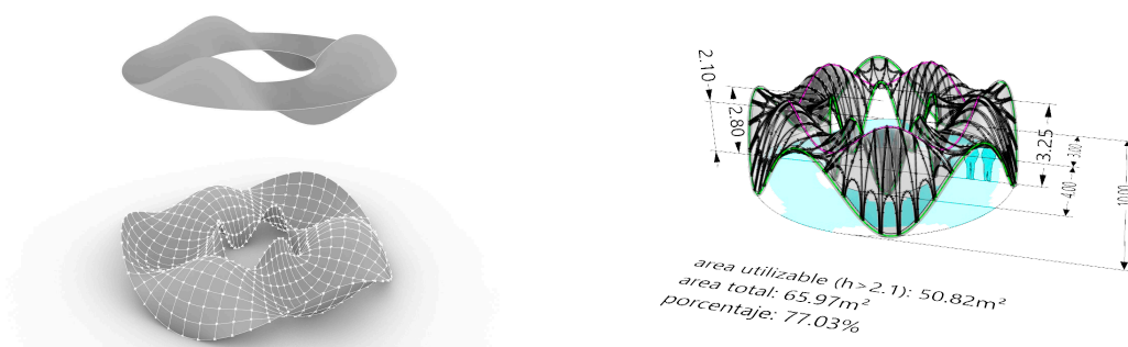
Figure 1,2: (left) Initial geometry diagram [R. Bolaños] (right): Geometric development and internal height analysis [R. Shiordia]
