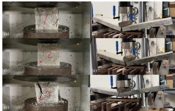
Figure 2: left compression test. (a) concrete; (b) FRC; (c) FRC with nonwoven at bottom. Figure 3: Right three-point bending test. (d) concrete; (e) FRC; (f) FRC with nonwoven at bottom.
