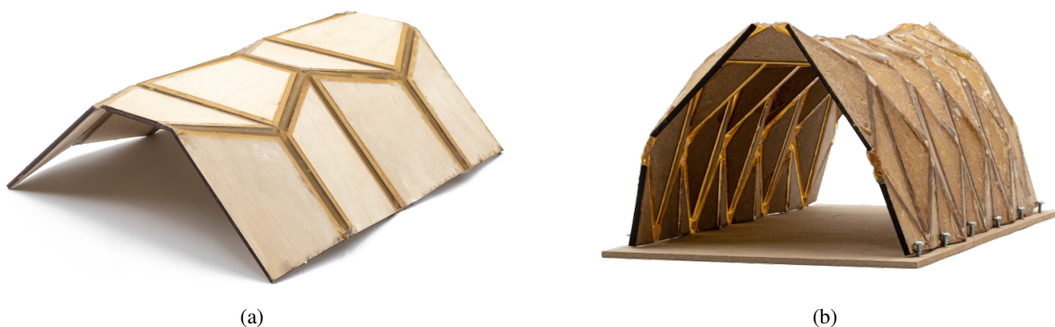
Figure 5: Linear kinetic joint structures:(a) chicken wire origami pattern; (b) Yoshimura origami pattern
