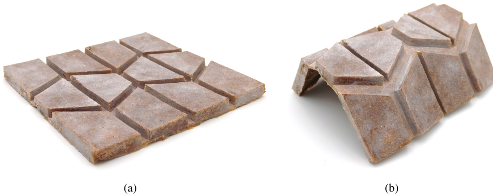
Figure 7: Monolithic foldable structure: chicken wire origami pattern
