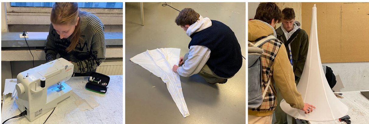
Figure 7: Fabrication of a membrane structure mock-up (left, centre) and the final shape of the mock-up (right)
