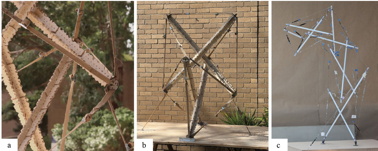
Figure 7: Prototype photos: (a) Detailed view of the full-scale prototype; (b) The full-scale prototype [Photographs: A. Pugnale]; (c) The 1:2 scale model with four kite modules [Photograph: M. Mack]
