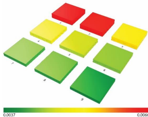
Figure 8: Visualization of the formwork material that would have been used for the production of each of the 9 concrete panels with traditional non-adaptable milled formworks. Red indicates a higher volume of material saved given the used adaptable formwork had the minimum height.
