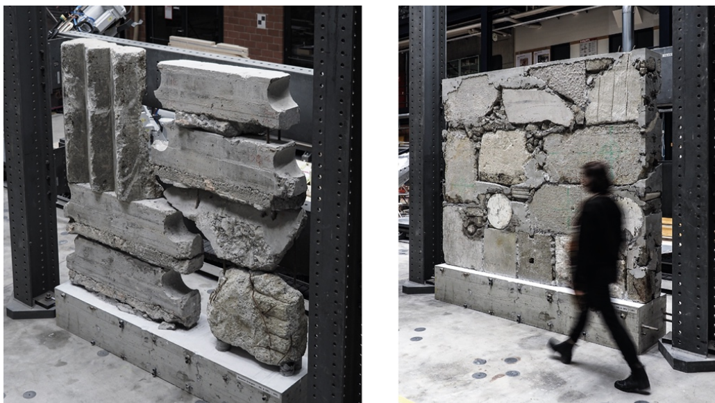
Figure 1: Demonstrators built by Grangeot et al. for the upcycling of concrete rubble into walls
