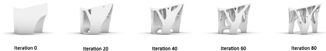
Figure 2: MV-BESO evolutionary history of snow pavilion
