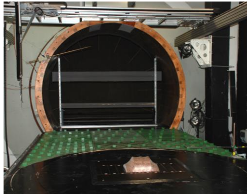
Figure 4: The 4-bay model and the ABL generators in the wind tunnel
