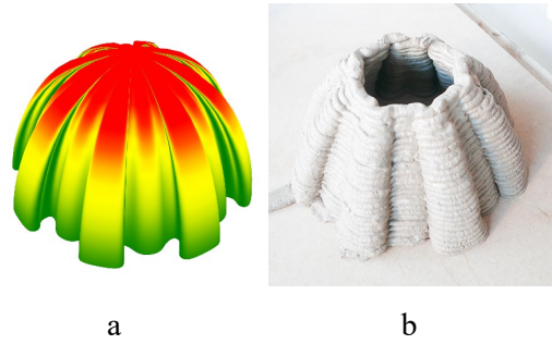
Figure 4 : (b)An example of a printable stoneware clay-based ribbed shell surface,(a)overhang angle simulation ( 40.50^\circ ).
