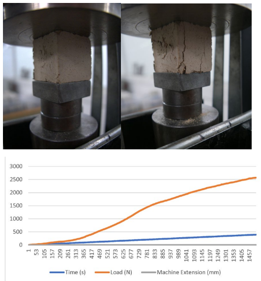
Figure 11: compressive strength test 1.028 N/mm 2
