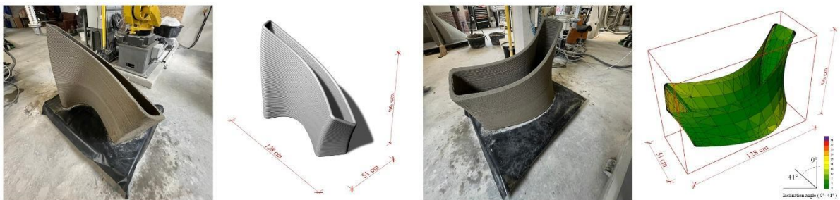
Figure 11: 3D print shell piece. A 3D concrete print of one of the pieces from the Shell type 3 – Cantilever, shown in Figure 9, demonstrating the ability of the GA to correctly split a shell into printable segments.
