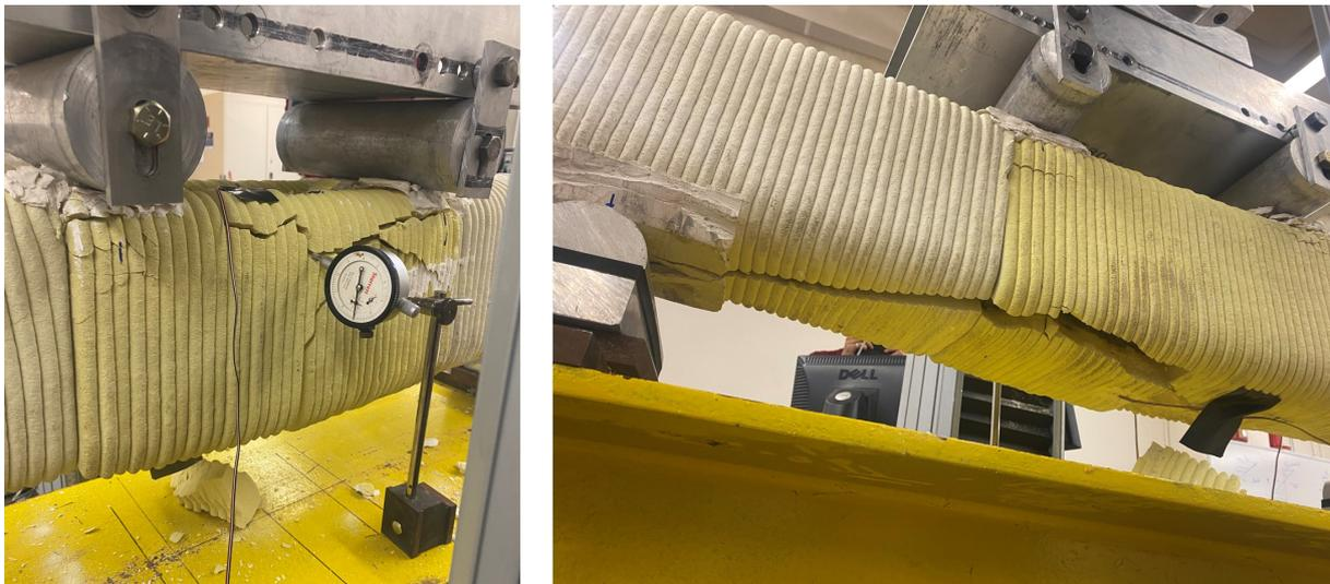
Figure 5: Failure mechanism under 4-point bending load
