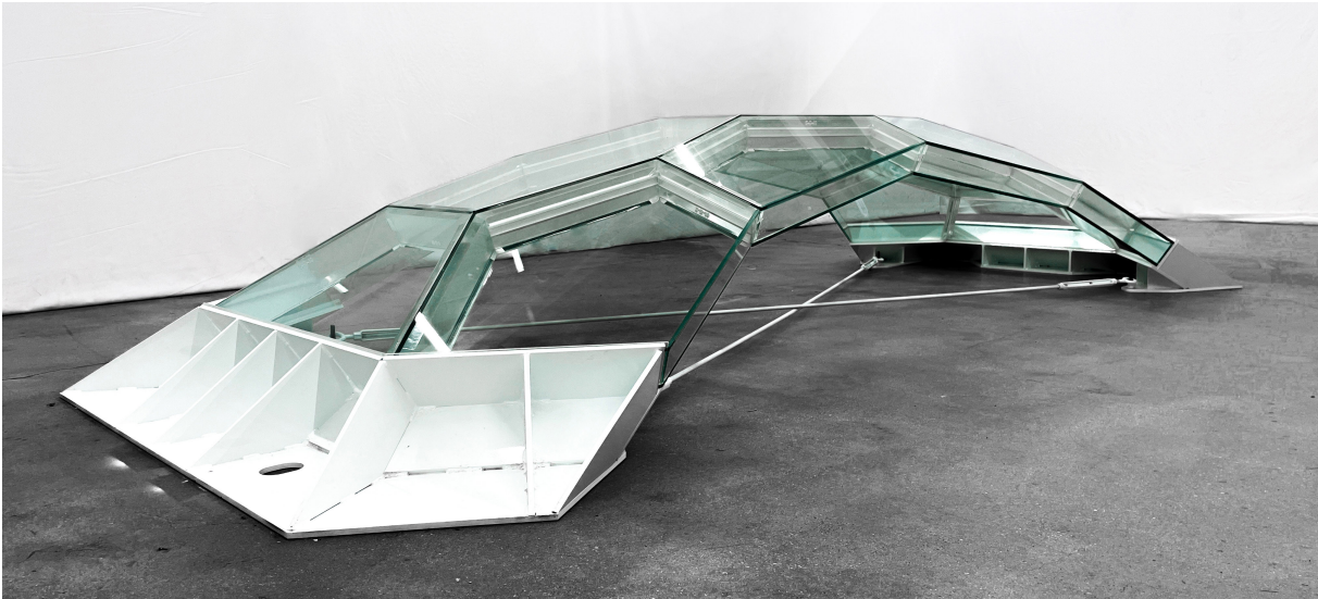
Figure 1. A 3m-span bridge prototype made of glass sheets [8].
