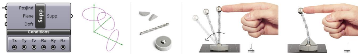
Figure 1: Supports and the 6 degrees of freedom demonstrated in Karamba 3D [4] - support component and graphical representation and with Mola components and forces demonstrating reactions [9].
