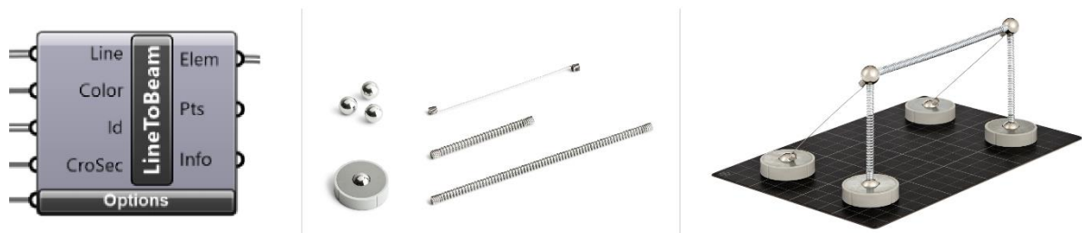
Figure 2: Component that converts lines to beam elements in Karamba3D [4] and with Mola components assisted to create rectangular frame and demonstrate connection types, reactions and deformations [9].
