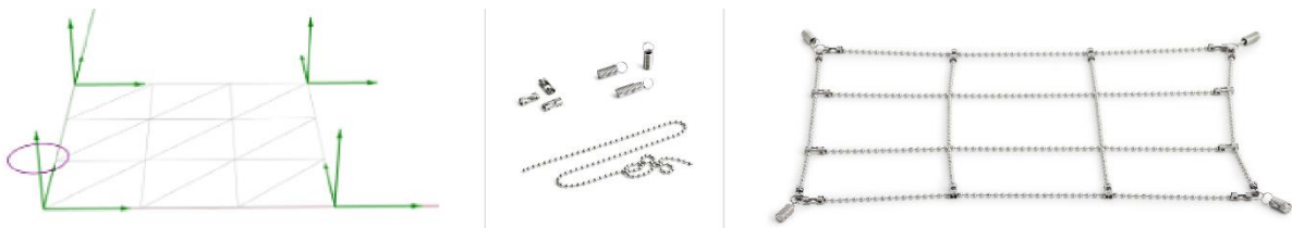
Figure 6: Simple shell element in Karamba3D prior to Kangaroo form-finding simulation and with Mola Structural Kit 3 components assisted using ground connections, cables and cable connection components [11].
