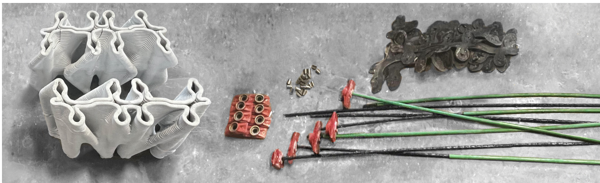
Figure 7: After testing, the modular funicular beam was disassembled efficiently and effectively. Since the beam was formed using ungrouted post-tensioning, the steel cables were readily removed from the concrete segments as well as all other construction materials, including the neoprene pads, post-tensioning anchors and wedges, all of which can be recycled.
