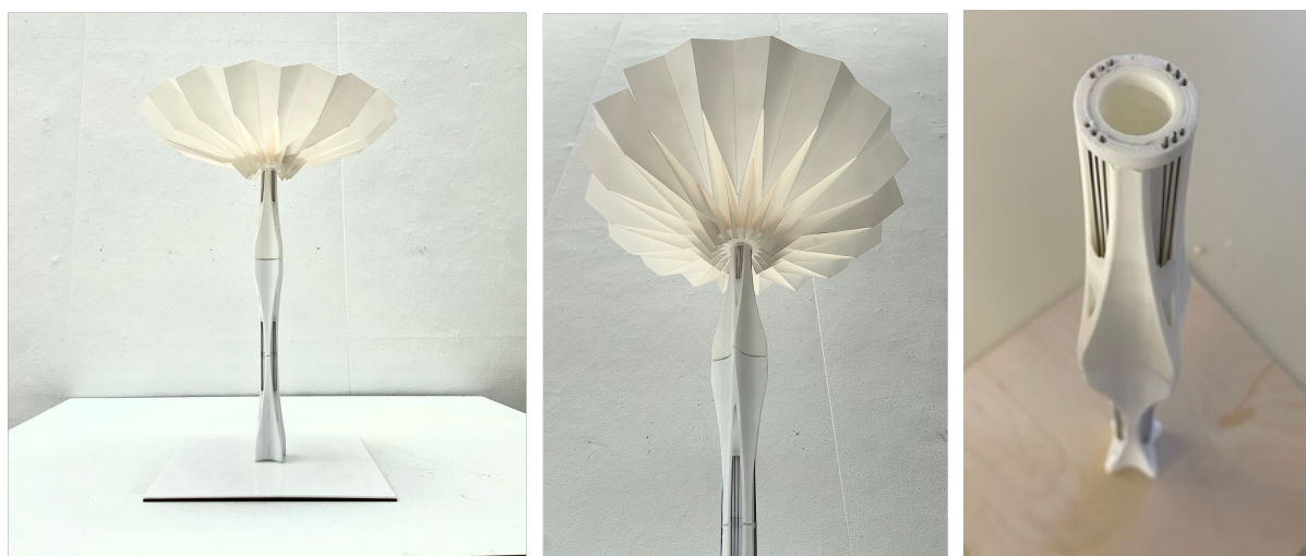
Figure 9: Scale model of the new prototype. 3D printed segmental columns with the folded membrane for sun shading and water collection (left) and detail of the segmental hollow column with the post-tensioning tendons (right). [Images: Tammy Feng, Liufei Zhu]
