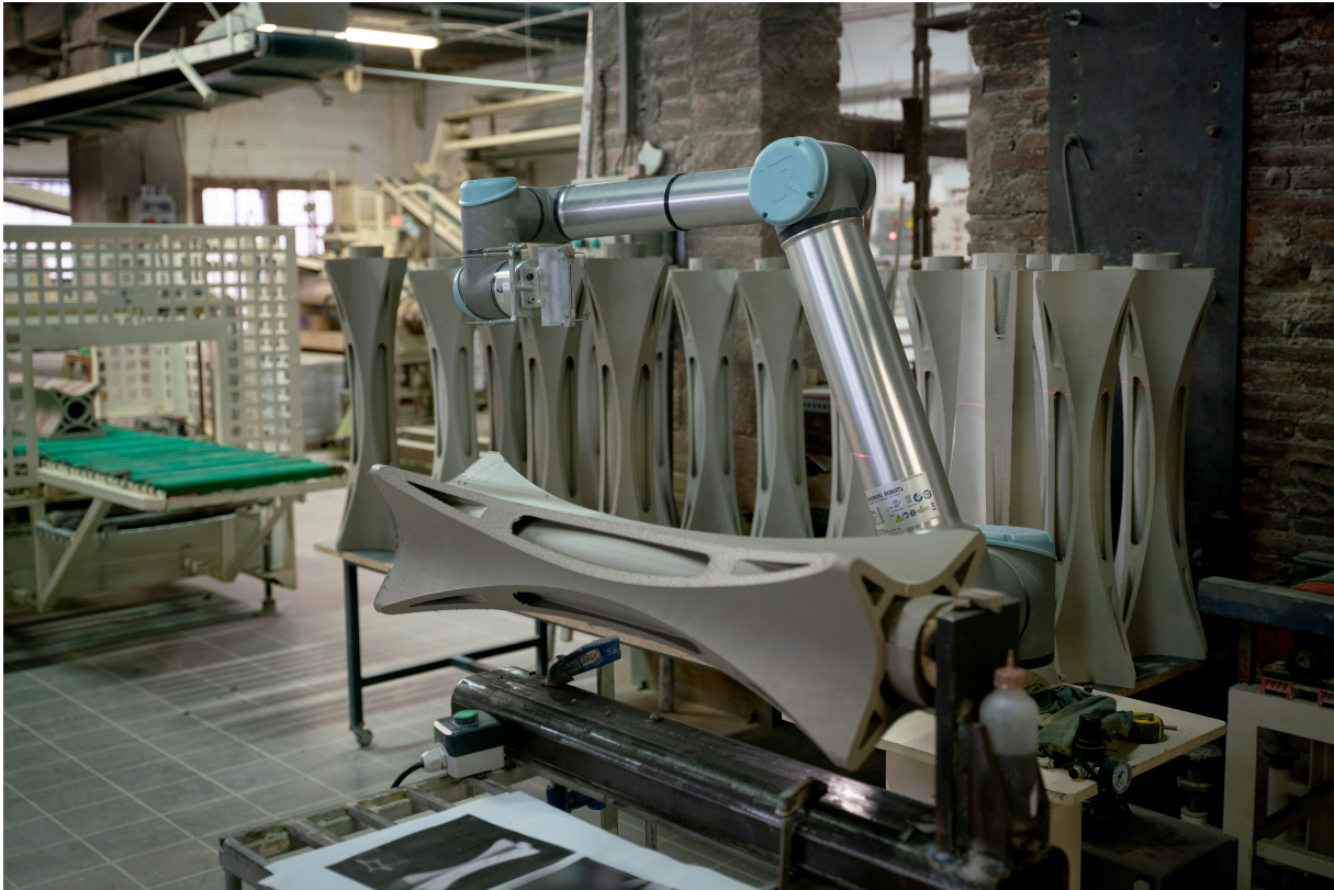
Figure 10: “Stem II” piece placed in the auxiliary structure for the precise robotic cuts and rotation [image: Frau Recerques Audiovisuals]
