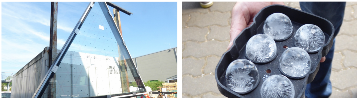
Figure 13: Hail stone impact test according to FM 4473.
