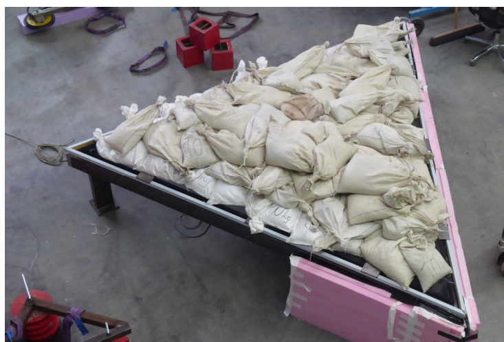
Figure 14: Static load test.
