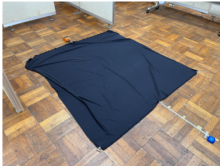
Figure 6: Tensile Force is measurement by pulling the each side of the cloth
