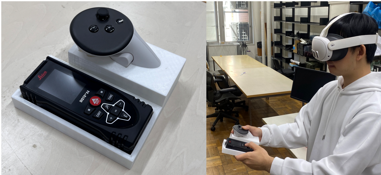
Figure 4 : 3D-printed laser distance meter and controller container
