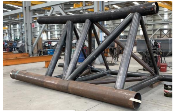
Picture 17 bottom of main flying mast fabrication. Picture 18 detail of ring section.
