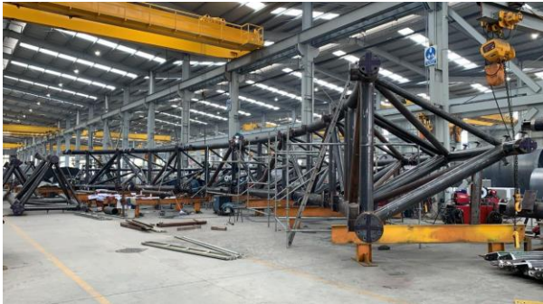
Picture 19 Pre-assembly of ring before ship to site. Picture 20 Pre-assembly of skirt before ship to site.
