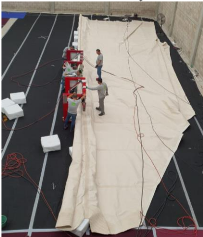
Picture 23 connecting main dome section. Picture 24 Welding reinforcements into main dome section.
