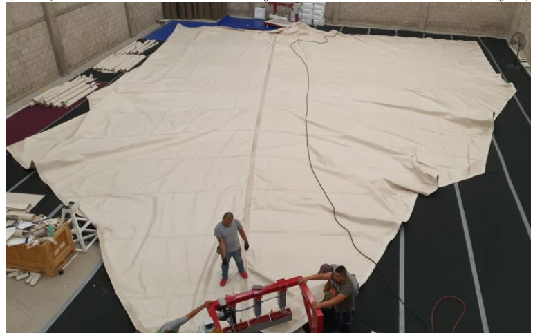
Picture 23 connecting main dome section. Picture 24 Welding reinforcements into main dome section.
