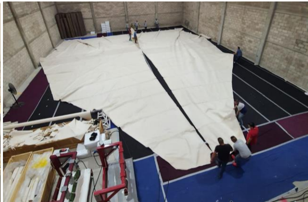
Picture 21 Fabrication of Skirt section (2-26). Picture 22 Fabrication of the main dome section (1 of 6)
