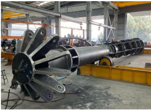
Picture 17 bottom of main flying mast fabrication. Picture 18 detail of ring section.
